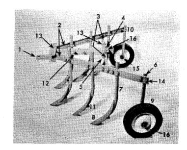
There is provision for a center shank which may be used for between row cultivating and furrowing. Remove one front shank and move the other into the slot between the center rail.
